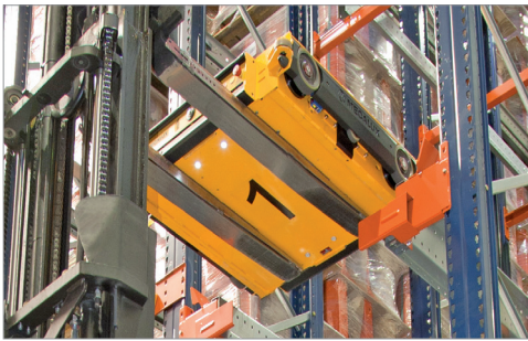
Locking system to ensure the shuttle is held in place on the forklift
